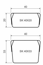
product description: they are used to separate individual types of lines in terms of electromagnetic compatibility is composed of two parts - canal and lid, both made of 0.55 mm thin galvanized sheet when mounting SK 40X33\_S, instruments with a great mounting depth cannot be used sections intended for fixing with PSK 1 are 250 mm apart
